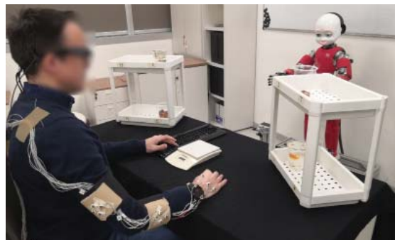
Fig. 1: View of the experimental setup with a volunteer in a rest position. The two shelves with the glasses on them, the motion capture markers and the iCub robot are visible
