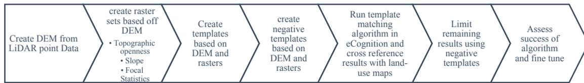
Figure 2: Steps involved in the use of template matching for the identification of mound features.
