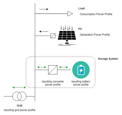
Figure 1: System Components of the AIT BESS sizing tool, before further developments in HYPER-RIDE.
