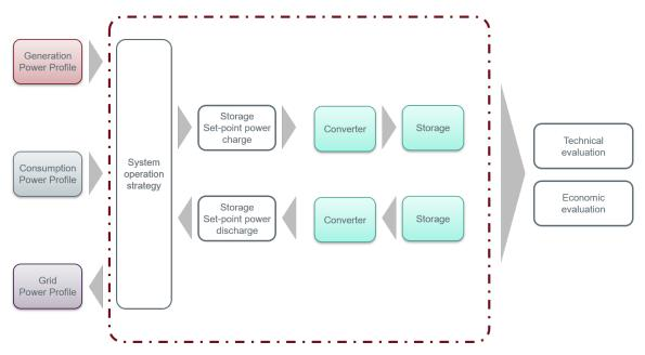
Figure 3: Schematic Component Sizing Tool components and component interaction.
