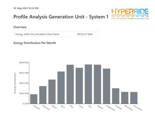
Figure 11: Partial profile analysis of a PV power with 50 kWp installed, facing south with 30 degree tilt.
