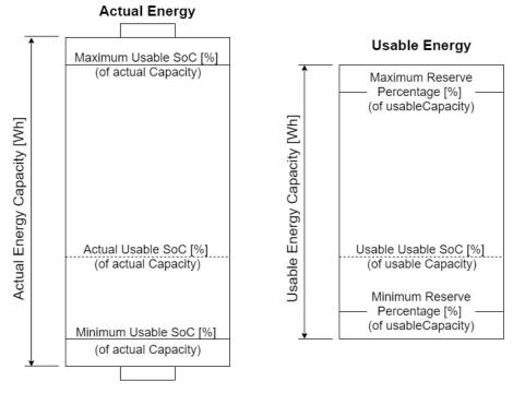
Figure 6: Visualisation of actual and usable BESS energy capacity (Kapeller, 2020).
