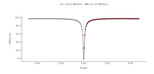
Figure 5: Converter Efficiency at 97 %.
