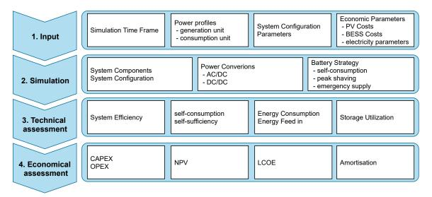
Figure 4: Simulation workflow.
