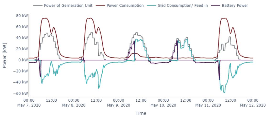
Figure 14: Partial analysis of the system application analysis, including a consumer, a generator and a BESS.
