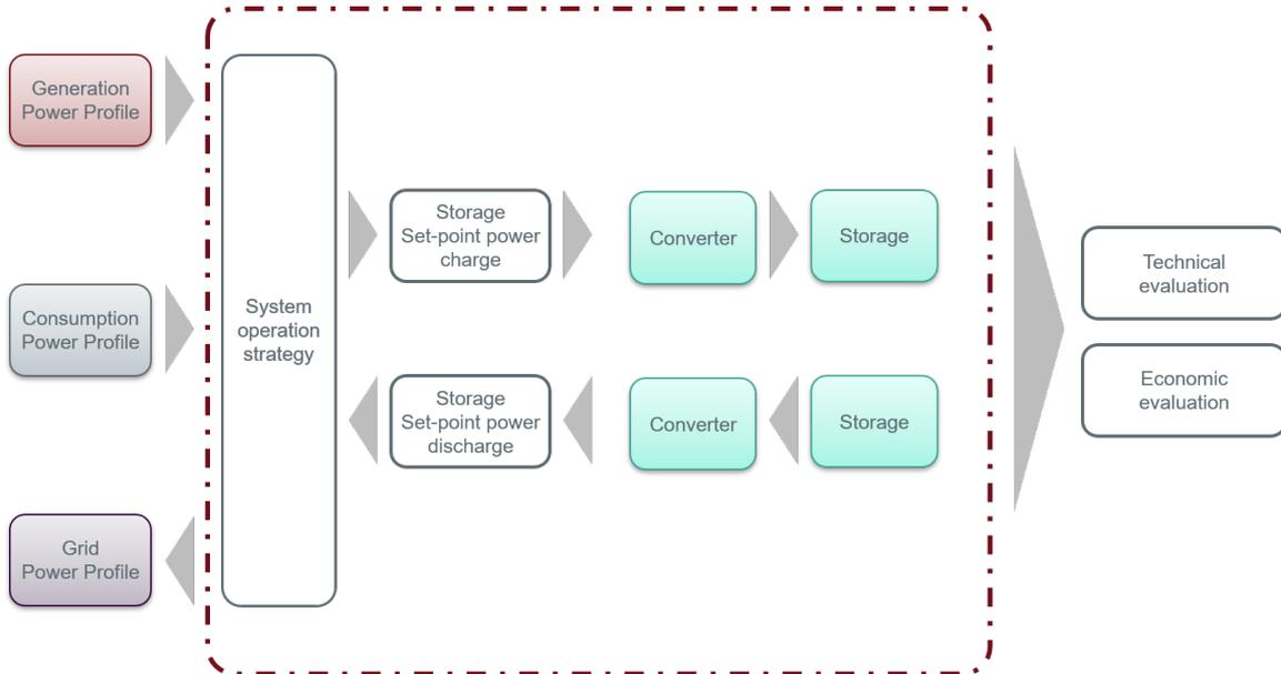
Figure 3: Schematic Component Sizing Tool components and component interaction.
