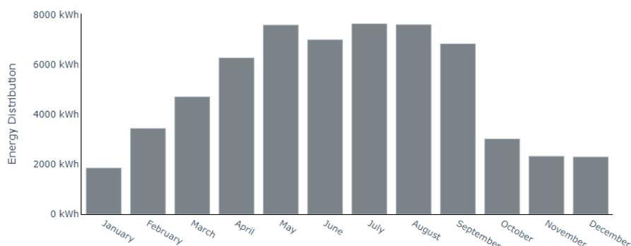
Figure 11: Partial profile analysis of a PV power with 50 kWp installed, facing south with 30 degree tilt.
