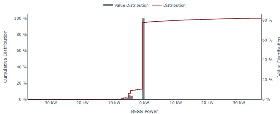
Figure 13: Partial analysis of a battery storage showing the storage system utilization.
