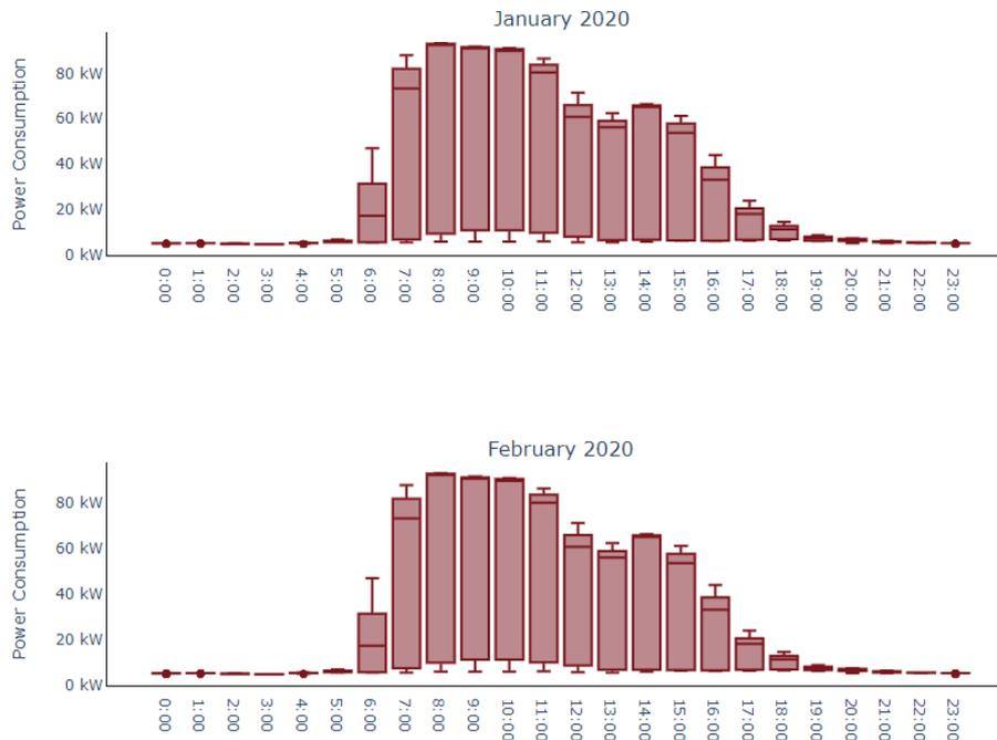
Figure 12: Partial profile analysis of an office building consumption profile with 192 500 kWh/a.
