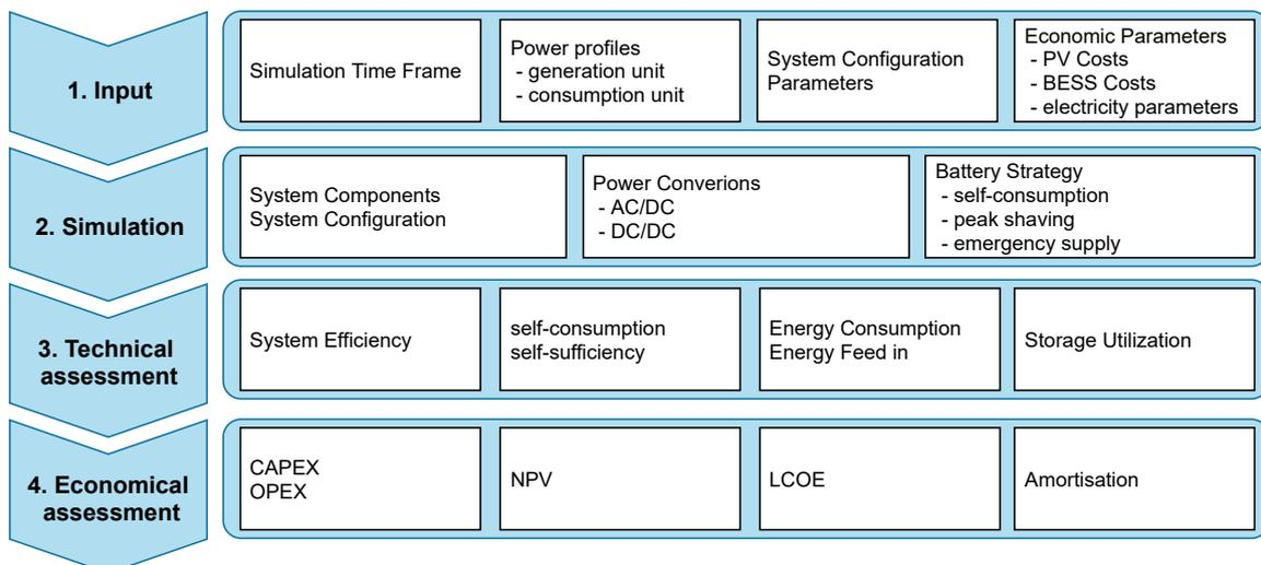
Figure 4: Simulation workflow.
