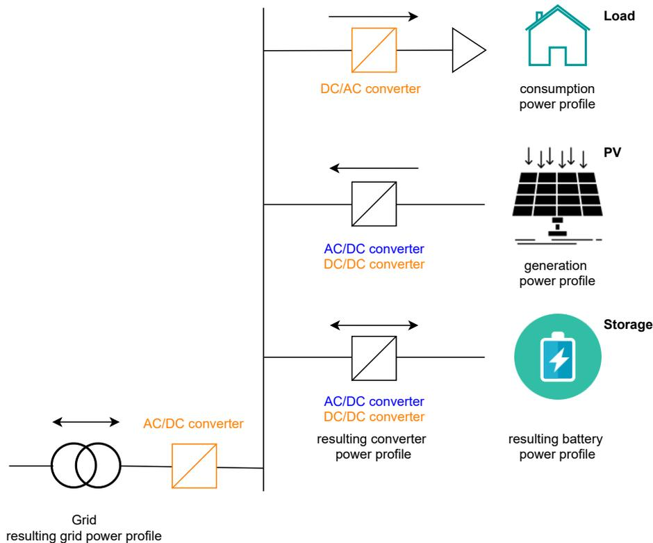
Figure 2: System Components of the Component Sizing Tool, as developed in HYPERRIDE.
