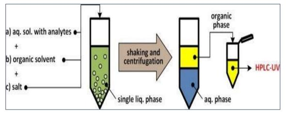
Fig 5: Salting Out Assisted Liquid-Liquid Extraction
