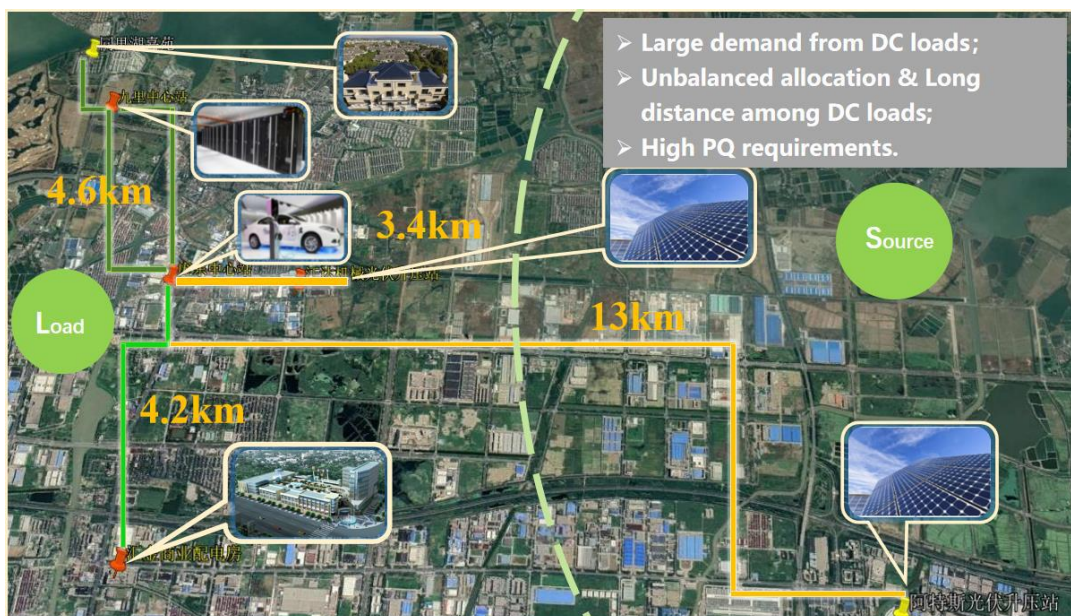
Figure 7: Medium-voltage DC distribution system demonstration project in Suzhou.
