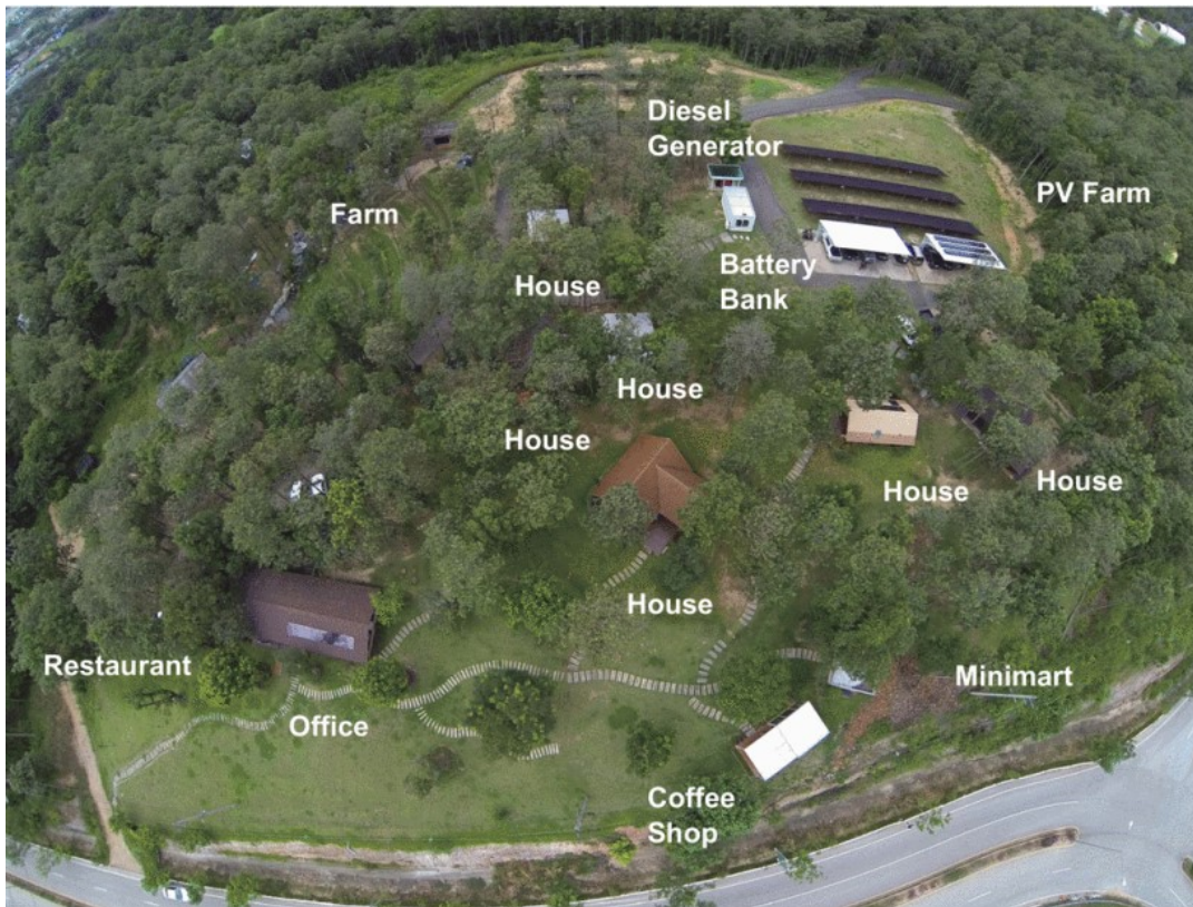
Figure 12: DC microgrid implemented in the smart community in Chiang Mai World Green City.
