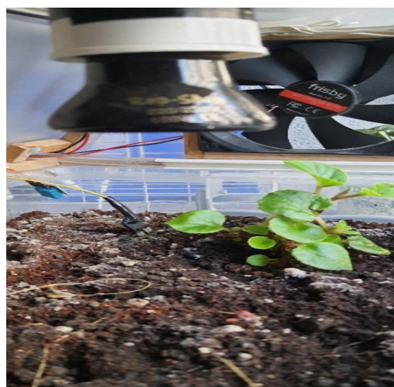
Fig. 2. Placement of the light and heater on the prototype
