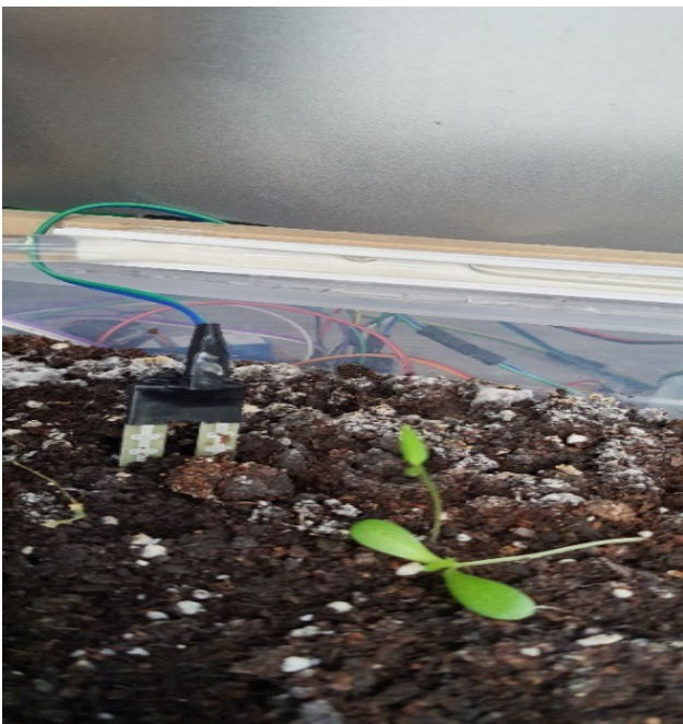
Fig. 4. Soil moisture sensors placed in the prototype
