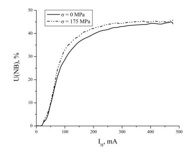
Фиг.4. Dependence of U (NB) in the tested samples on the magnetizing current I<sub>H</sub> in the sample without load  $\sigma = 0$  MPa and with load  $\sigma = 175$  MPa.
