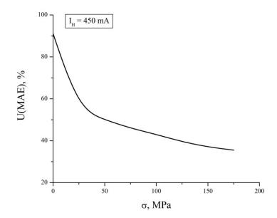
Fig.7. Dependence of the voltage U (MAE) of the magnetoacoustic emission, at magnetizing current  $I_H = 450$  mA on the tensile stresses  $\sigma$  in the tested sample.
