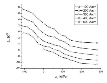
Fig. 1 Dependence of  $\lambda$  and  $\sigma$  at different values of magnetic field strengths for steel 45.
