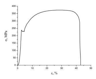
Fig. 3. Tensile diagram for sample steel grade S235
