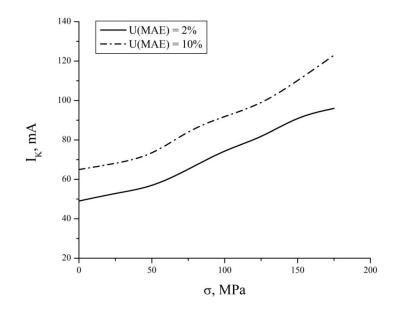
Fig.6. Dependence of the critical magnetizing current  $I_K$  at which the registration of U (MAE) starts at the level of 2% and 10% of the mechanical stresses  $\sigma$  in the sample
