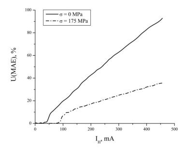
Fig.5. Dependence of the voltage of magneto-acoustic emission U (MAE) in the tested samples on the change of the magnetizing current I<sub>H</sub>, without load  $\sigma = 0$  MPa and with load  $\sigma = 175$  MPa.
