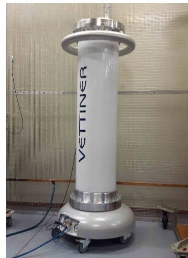
Figure 3 HV capacitor with 4 \mu\text{F}/\text{F} voltage dependence up to 230 kV.
