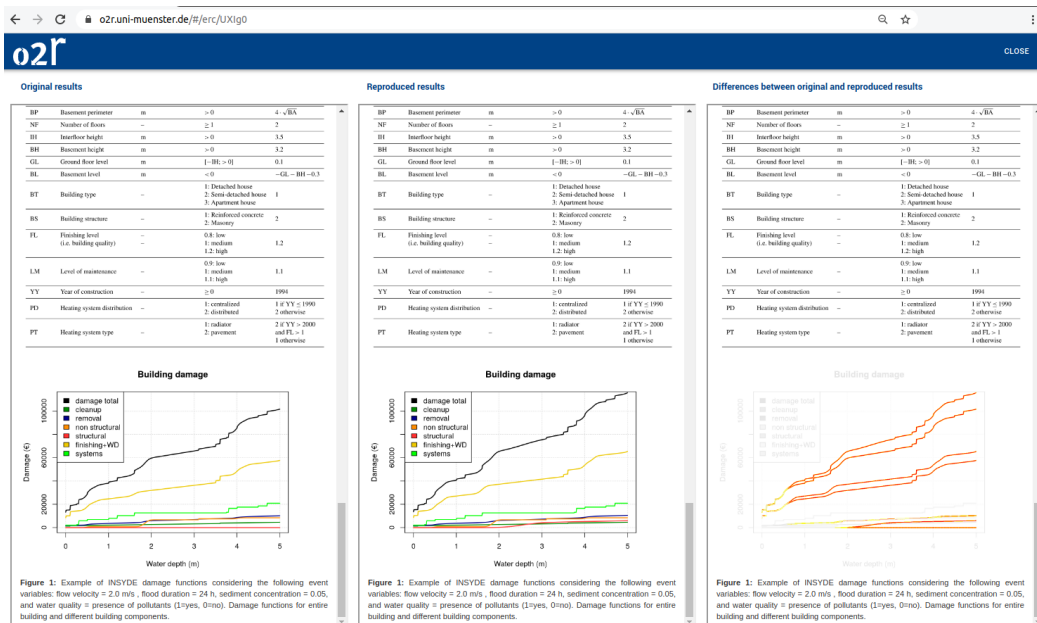
Fig. 6. Screenshot of the ERS user interface showing the result of a failed job execution due to differences in a figure. Left column: display file provided by the author; middle column: display file generated by the ERS; right column: display file with highlighted difference generated by erc-checker.
