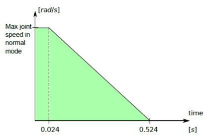
The green area below the ramp is the allowed speeds for a joint during braking. At time 0 an event (emergency stop or safeguard stop) is detected at the safety processor. Deceleration begins after 24 ms.
