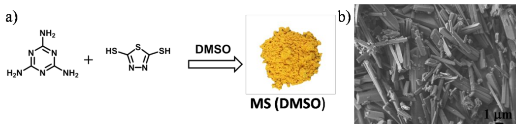
Figure S1. a) Schematic illustration of the formation of MS (melamine-bismuthiol) supramolecular assemblies. b) SEM image of the as-synthesized supramolecular MS (DMSO) assembly.
