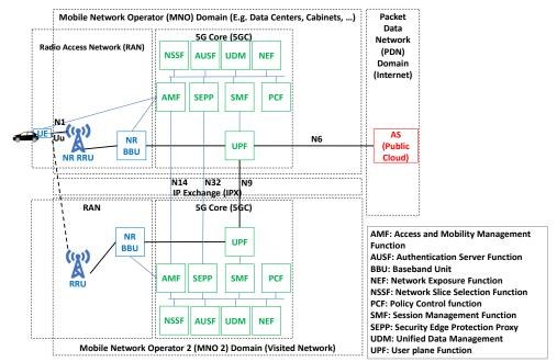
Figure 2. Standalone 5G New Radio home-routed roaming architecture with N14 interface between AMFs
