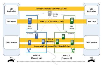
Figure 1. Overview of technologies and entities required to deliver 5G-enabled cross-border CCAM services
