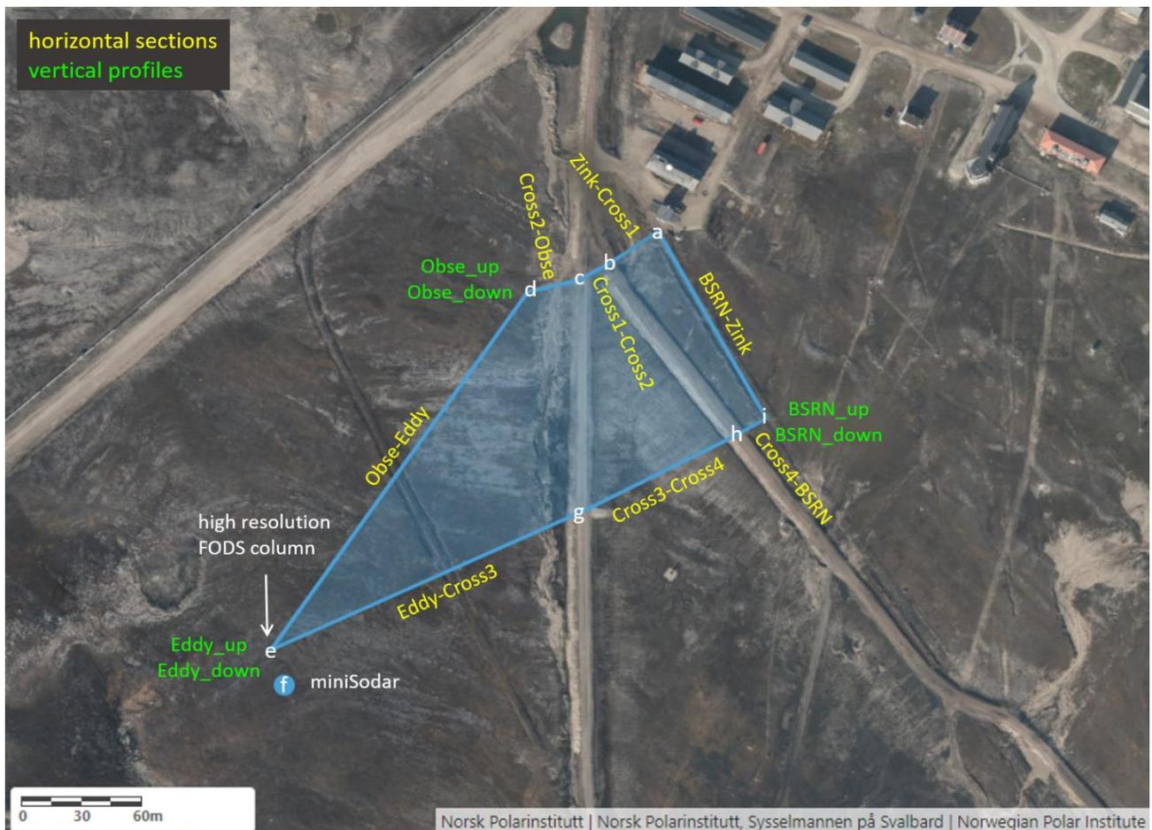
Figure 2. Setup south of Ny-Ålesund. The labels are the section names of the fiber optic Array (see *File overview*). The letters a-i mark crucial points with their coordinates listed in table 1. The map source is Svalbardkartet ([geokart.npolar.no/Html5Viewer/index.html?viewer=Svalbardkartet](http://geokart.npolar.no/Html5Viewer/index.html?viewer=Svalbardkartet)).
