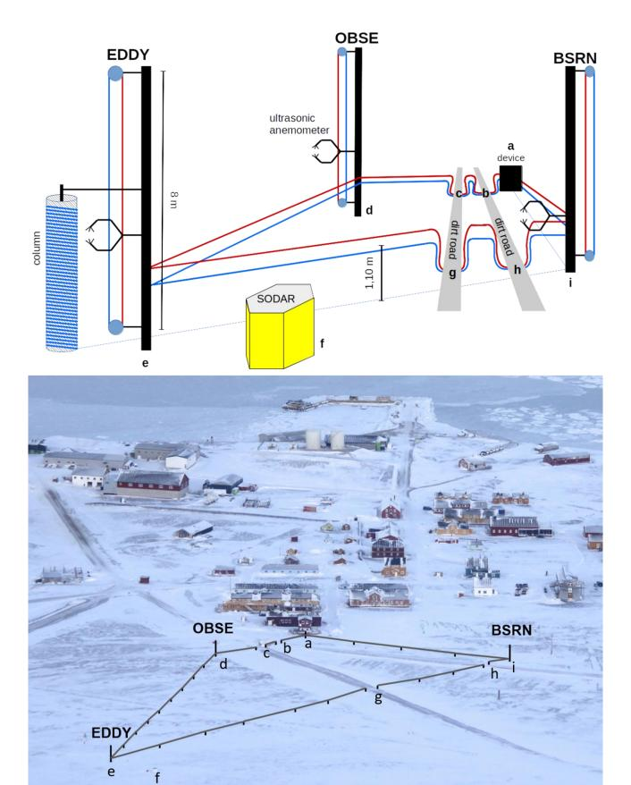
Figure 3. Schematic setup and picture of the setup from the Zeppelin mountain from south. The fiber-optic array has a length of 700 m. The coordinates of the characteristic points a-i of the schematic setup can be found in the Table 1. Photo credit: Harald Sodemann (UBergen, Norway).
