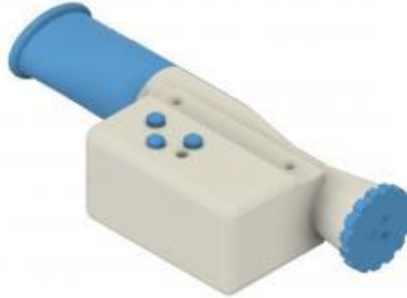
Spirotroller gaming [J] Controller measuring the flow and pressure, 3d-printed, Bluetooth, three buttons
