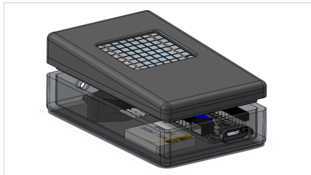
Led box [C] Controller measuring the expiratory pressure, 3d-printed, Bluetooth and USB, 8x8 LED matrix
