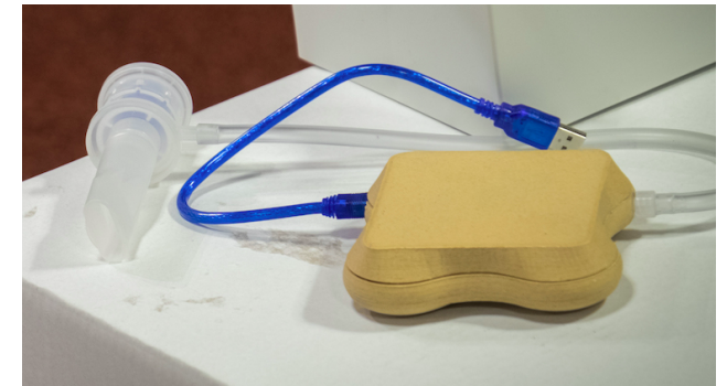
3D organic box [B] Controller measuring the expiratory pressure, 3d-printed, USB, 1 LED
