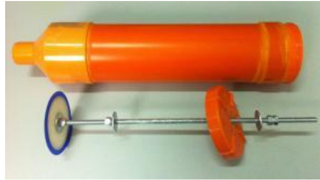
Calibration syringe [E] 3 liter syringe for calibration
