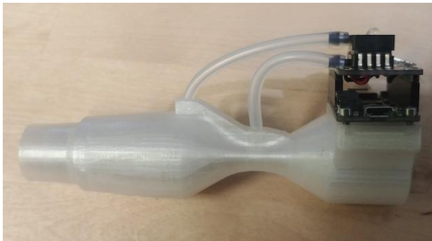
Spirotroller [G] Game controller measuring the expiratory flow, 3d-printed, Bluetooth and USB, one button
