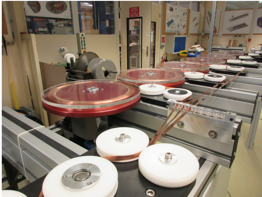
Figure 6.23 View of the multi-spool winding table assembled in the TE-MS-C-MDT laboratory
