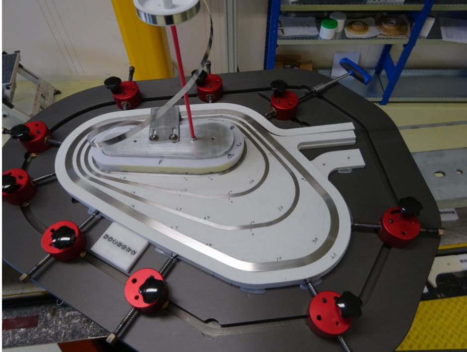
Figure 6.30 First layer of GaToroid dummy prototype, wound in stainless steel tape on glass-filled nylon spacers (white), together with the winding plate (black) and the tooling (red)
