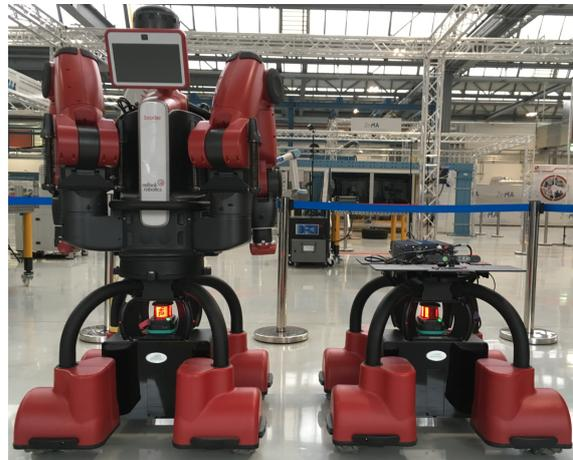
**Fig. 3.8.:** Mobility Base with and without Baxter Robot mounted on top
