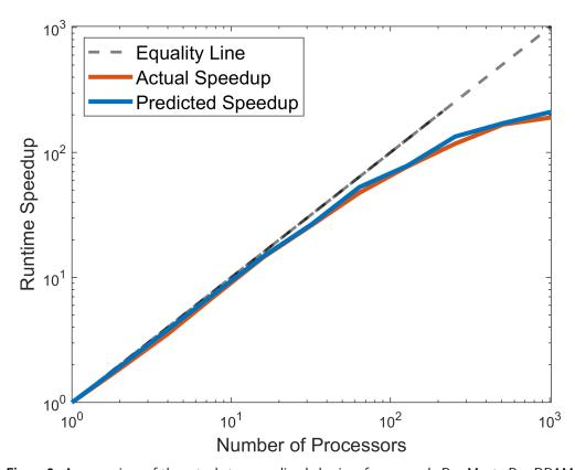
**Figure 2:** A comparison of the actual strong scaling behavior of an example ParaMonte-ParaDRAM simulation from 1 to 1088 processors with the strong-scaling behavior predicted during the post-processing phases of the corresponding individual ParaDRAM simulations. The data used in this figure is automatically generated for each parallel simulation performed via any of the ParaMonte samplers. The black dashed line represents the perfect parallelism.
