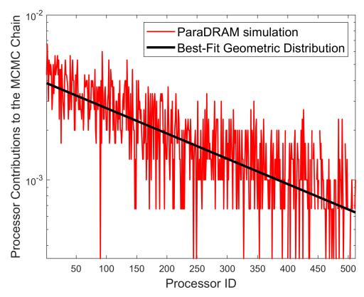
**Figure 1:** An illustration of the contributions of 512 Intel Xeon Phi 7250 processors to a ParaMonte-ParaDRAM simulation parallelized via the Fork-Join paradigm. The predicted best-fit Geometric distribution from the post-processing phase of the ParaDRAM simulation is shown by the black line. The data used in this figure is automatically generated for each parallel simulation performed via any of the ParaMonte samplers.
