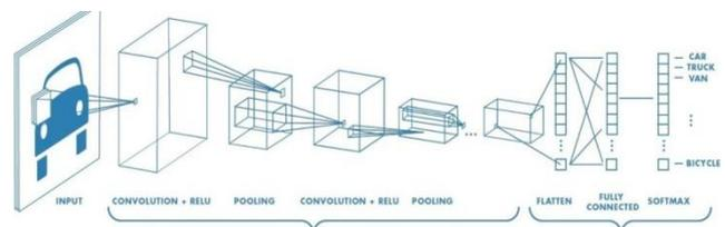
Fig. 9 Block diagram of Convolutional Neural Network (CNN)
