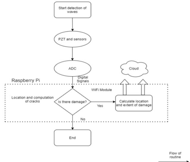
Fig. 7 Schematic flow of a routine SHM using IoT paradigm
