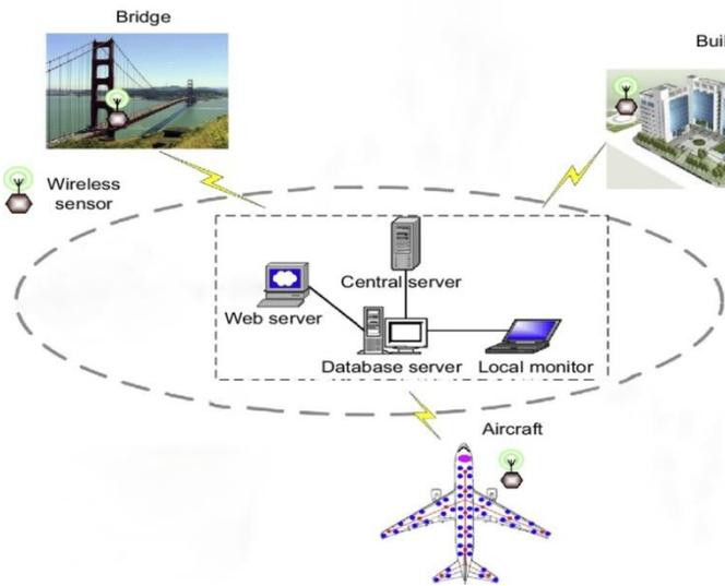
Fig. 6 Schematic Diagram of Wireless Sensor Networks in Structural Health Monitoring
