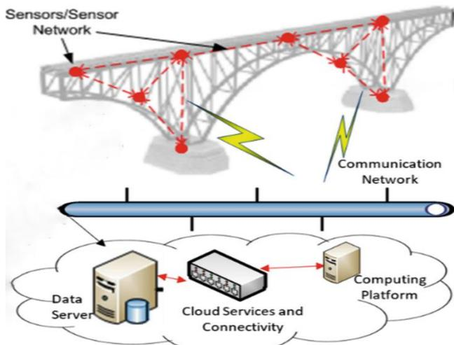
Fig. 8 The Cyber-Physical Bridge Monitoring System for SHM
