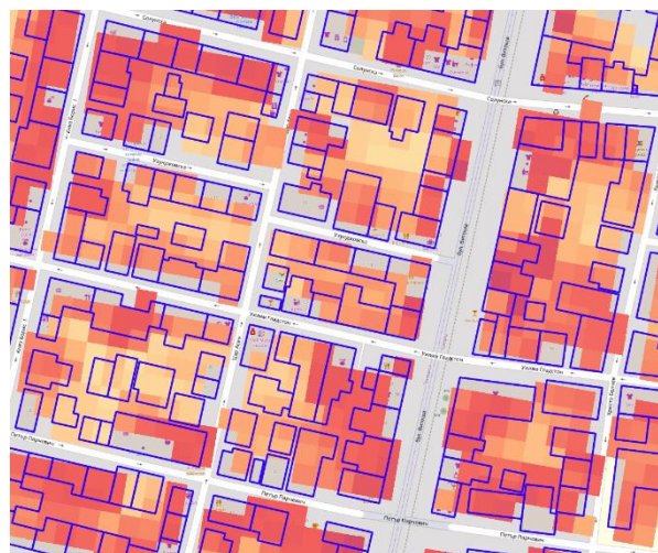
Figure 32. Illustrations of the two datasets used for the 3d building model. The blue lines indicate the ground plan of the buildings according to OpenStreetMaps data, while the yellow-to-red colors indicate the building height according to the 10m resolution UrbanAtlas dataset. Background image: OpenStreetMaps.org.
