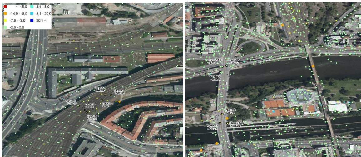
Figure 26. Stable points with terrain/surface movements subsidence measurements, classified by velocity of movements in urban area.
