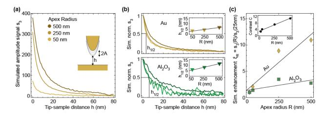
Figure 6: Numerical simulations considering tip modulation and signal demodulation. (a) Simulated  $s_3$  approach curve for different tip apex radii. Sample is gold. (b) Simulated normalized approach curves for Gold (top) and Alumina (bottom) samples. Insets show the distance at which the signal decreases to half maximum (solid lines are linear fits). (c) Simulated signal enhancement for Gold and Alumina samples. Inset: contrast calculated from simulation (solid lines are linear fits).
