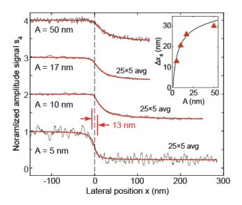
Figure 8: Pushing the resolution with sharp and long tips. Line profiles across the metal/dielectric boundary of the test sample recorded with a W-tip with R = 6 nm at varying tapping amplitude A (avg: number of averaged scans of which each one was smoothened with an average filter over 5 adjacent data points). Inset: Resolution  $\Delta x$  as function of tapping amplitude.
