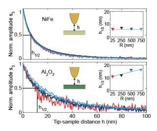
Figure 3 : Approach curves for tips with different tip radii recorded on the metallic NiFe (top) and dielectric  $Al_2O_3$  (bottom). Insets show the distance  $h_{1/2}$  at which the signal drops to half of its maximum.
