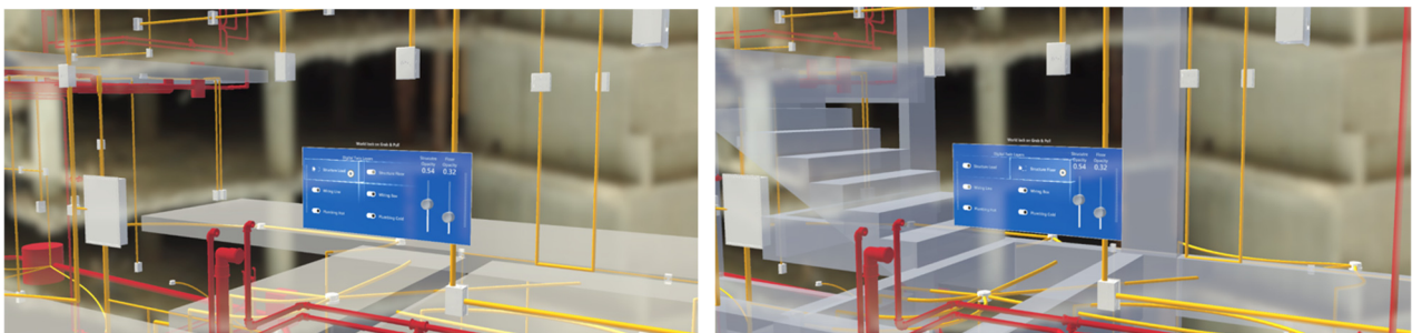
Figure 17: Left: Floor layer is switched off. Right: Load-bearing structure layer is switched off
