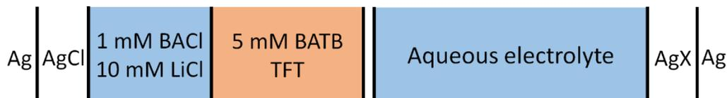
**Scheme 1.** The general configuration of the four-electrode electrochemical cell used for cyclic voltammetry (CV) and AC voltammetry measurements. Only the aqueous electrolyte composition was varied between studies. The organic electrolyte solution was always  $\alpha,\alpha,\alpha$ -trifluorotoluene (TFT) containing 5 mM bis(triphenylphosphoranylidene)ammonium tetrakis(pentafluorophenyl)borate (BATB).
