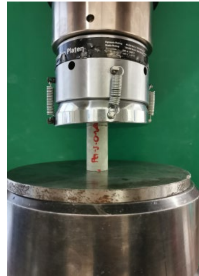
Figure 8: UCS testing apparatus with rock sample during loading.
