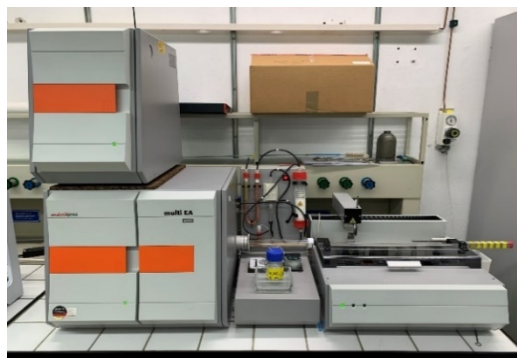
Figure 13: Left: Determination of carbon content with multi EA 4000 device, right: close-up of TIC determination with H 3 PO 4 .
