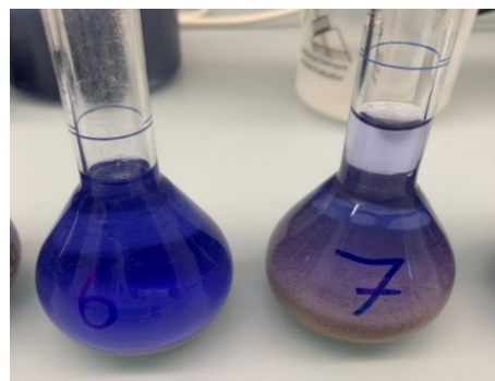
Figure 3: Left sample depicting a low CEC compared to high CEC on right sample.
