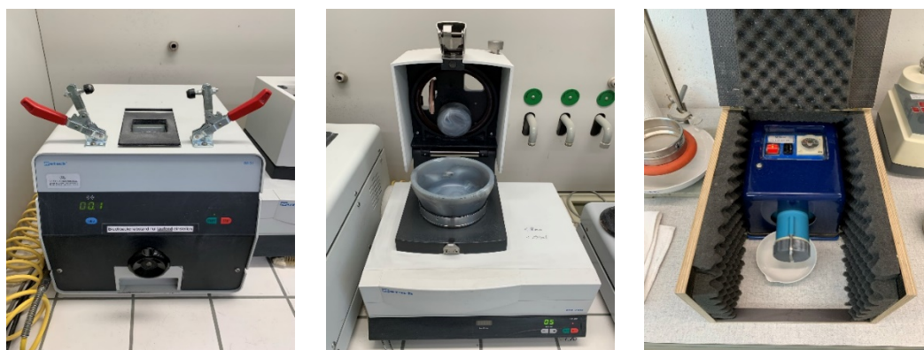
Figure 1: Overview of mills used for sample preparation. Left: jaw crusher for fraction <400 µm, middle: agate mill for fraction <63 µm, right: vibrating McCrone mill for fraction <20 µm.
