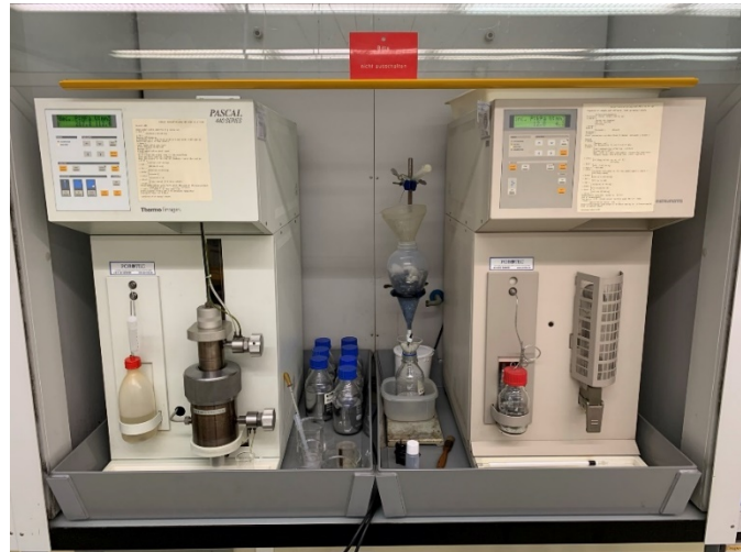
Figure 11: Low- and high-pressure chambers to analyse porosity and pore size distribution. Right: low-pressure device for mercury intrusion, left: high-pressure device to further induce the mercury into nanometer pores using high-pressure
