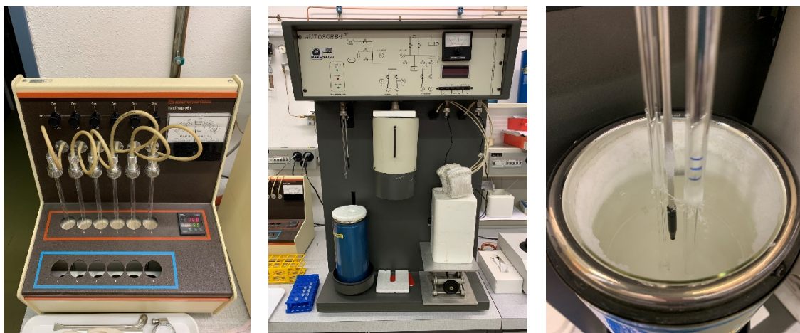
Figure 8: Left: VacPrep 061 vacuum pump used for sample degassing, middle: Quantachrome Autosorb-1 device for measuring specific (outer) surface, right: close-up of liquid nitrogen tank, in which sample is immersed.
