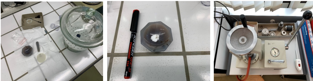
Figure 5: Tools required for FTIR sample preparation. Left: agate mortar, funnel and desiccator (for sample conservation), middle: 1 mg of sample mixed with 199 mg KBr, right: pressing apparatus applying 10 tons onto the sample resulting in the pressed KBr pill.
