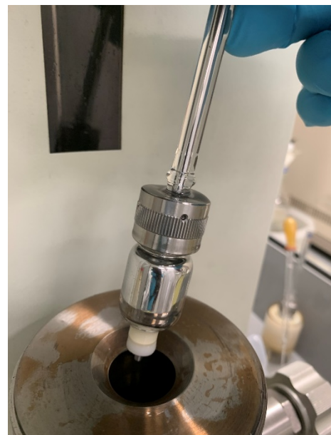
Figure 12: Transfer of mercury injected sample from low-pressure to high-pressure device.
