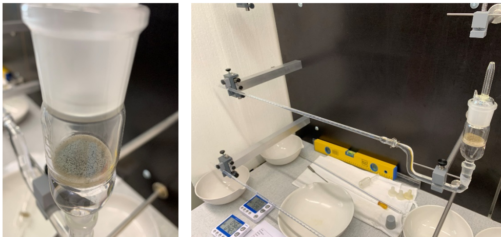
Figure 10: Left: close-up of sample burette with sample powder during water uptake, right: full Enslin-Neff apparatus including scaling burette to read absorbed water in ml.
