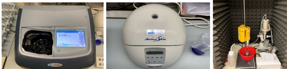
Figure 4: Required measurement devices for CEC determination. Left: Spectral-Photometer DR 6000 by Hach Lange, middle: Eppendorf MiniSpin centrifuge, right: ultrasonic UP 200H.
