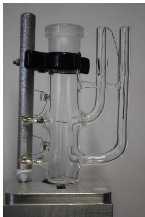
Figure S1. Schematic and image of the glassware of a four-electrode electrochemical cell. The aqueous and organic counter electrodes (CE) are platinum wires and the aqueous and organic reference electrodes (RE) are Ag/AgCl wires. The liquid-liquid interface is always situated mid-way between the two Luggin capillaries. The organic phase is a halogenated solvent (either \alpha,\alpha,\alpha -trifluorotoluene or 1,2-dichloroethane) with a greater density than water and therefore is the bottom layer.
