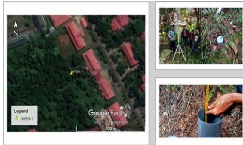
Figure 3. Placement and installation ardupeat
