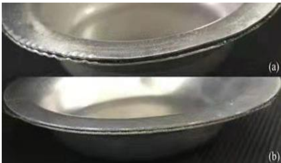
Figure 1.7: Delamination in the specimen [4]
