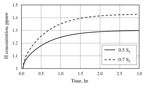
**Figure 11.** Hydrogen concentration on the surface facing the probe during the test with different maximum tensile stresses applied to the specimen (Sy: Yield strength).
