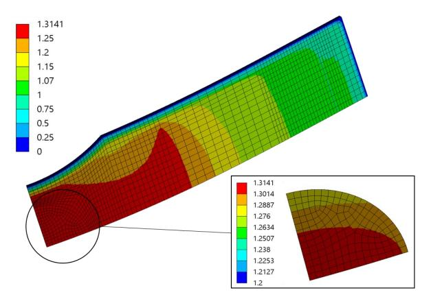
**Figure 8**. Hydrogen concentration on the tensile side of the specimen at the end of the test, simulation ran starting from a uniform initial concentration of 1 ppmw.
