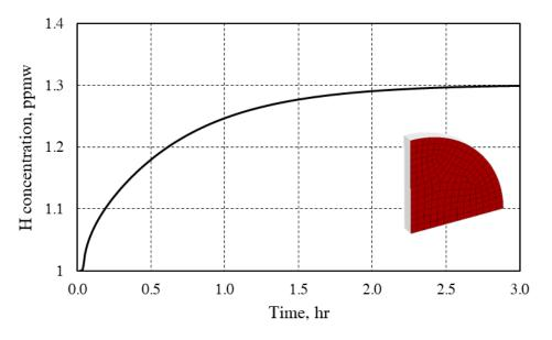
**Figure 9.** Evolution of the hydrogen concentration on the surface facing the probe, during the mechanical test.
