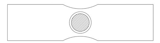
Figure 2. Desorbed region of the specimen (dashed area).
