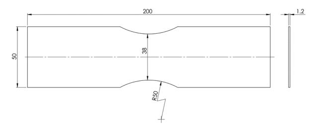
Figure 1. Drawing of the specimen.
