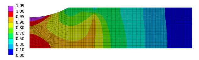
Figure 6. Hydrostatic stress distribution on the specimen tensile surface (stresses normalized with respect to the maximum value occurring in the central region).
