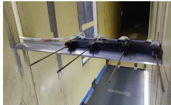
Figure 12. Four, Seven-Holes Probes mounted on the wake traverse system, 1350 [mm] downstream from the wing rotation axis and spaced 9 and 12 [cm] apart.
