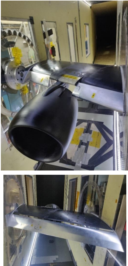
Figure 5. Front (top) and rear (bottom) views of the SSM (or GSM) installed at the TAU Knapp-Meadow WT at TAU.
