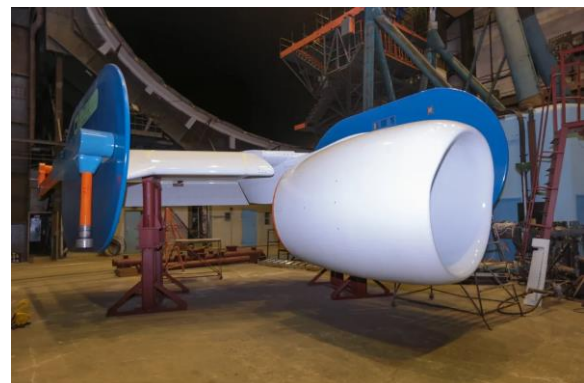
Figure 4. The LSM (termed also BFM) at the T-101 WT in TsAGI during the INAFLOWT project. The span and the chord of this model are larger than 5m.
