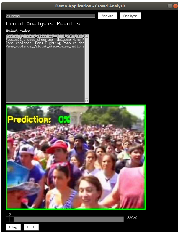
Fig. 5. A non-violence related example of the proposed framework user interface after completing the analysis of three videos. On the top, a list of the analyzed videos is depicted. On the bottom, the outcomes of the analysis for the corresponding selected video are shown.
