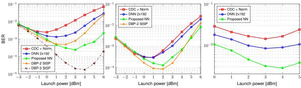
Fig. 2: Numerical test for 6×80 km LEAF Fig. 3: Numerical test for 6×80 km SSMF Fig. 4: Field trial for 612 km SSMF
