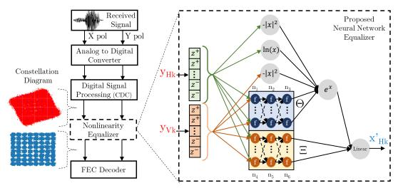
Fig. 1: Structure of reveicer with the architecture of the proposed neural network.
