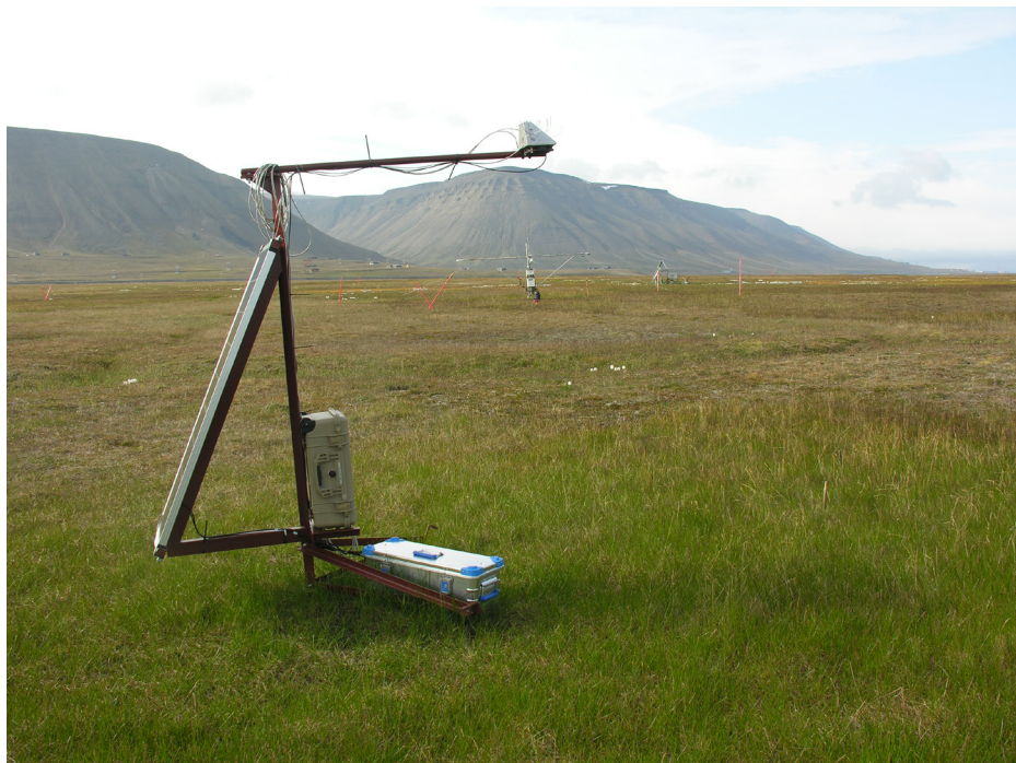
Figure 5: Sun-Induced measurements by the spectroscopy system FLoX. The FLoX-system (foreground) is established near and within the footprint of the Eddy-Covariance station (in background) in Adventdalen (Photo: Lennart Nilsen).
