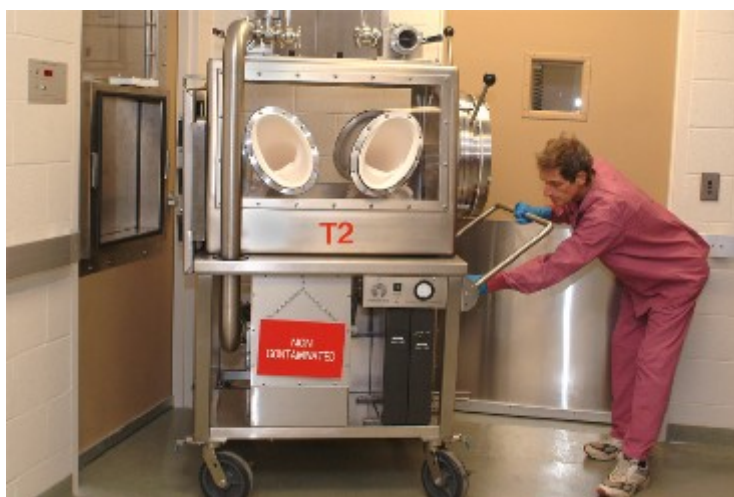
Example of a mobile Class III BSC (Biosafety Cabinet)—suitable for a BSL-4
