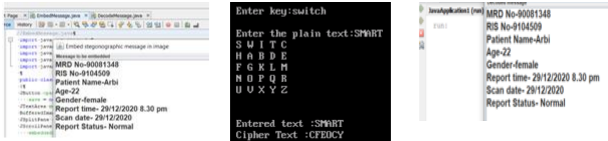
(a) Patient's Information as Plaintext (b) Playfair Ciphertext (c) Retrieved Patient's Information
