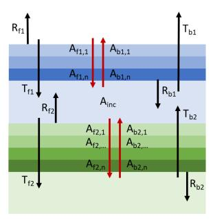
First, reflectance is derived by following the ray interactions (see above figure) within the joined stack. The total reflectance is then the sum over the individual paths:
