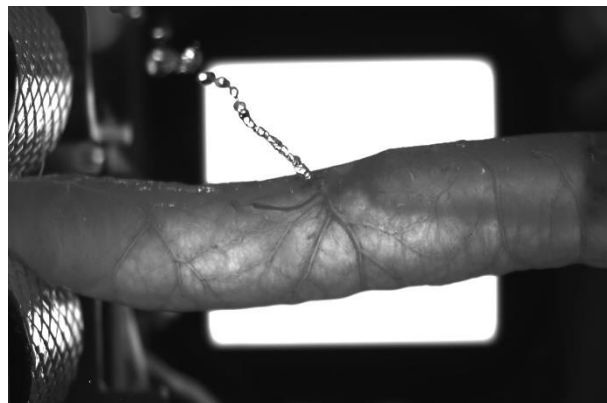
Figure 1: Grayscale image of a water-filled pig intestine in the SelectiCa machine, lit by back lighting, showing a fountain produced by a small hole.
