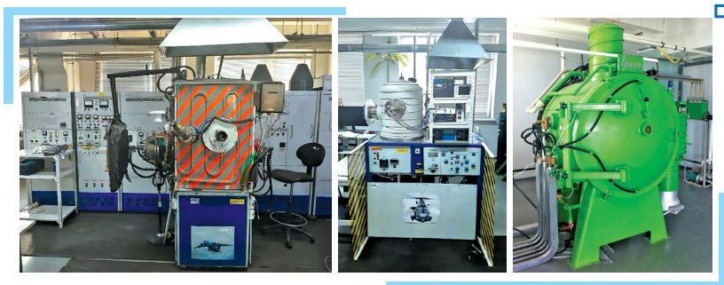
□ Fig. 2.1 Avinit vacuum-plasma automated cluster
