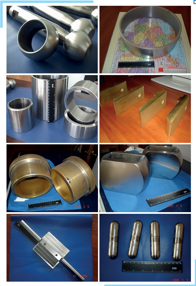
■ Fig. 5.1 Elements of mechanisms of steam distribution and steam regulation of steam turbines working in hinged connections and sliding bearings with wear-resistant antifriction nanocoatings Avinit
