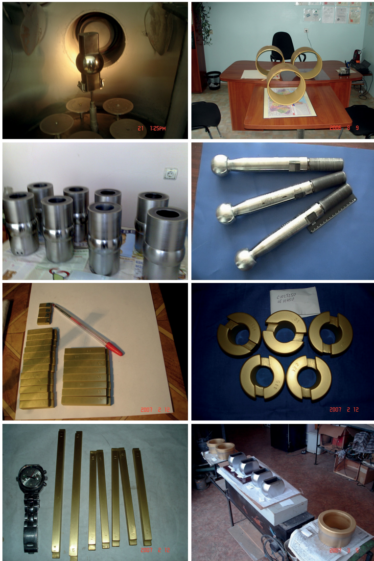
■ Fig. 5.2 Elements of mechanisms of steam distribution and steam regulation of steam turbines working in hinged connections and sliding bearings with wear-resistant antifriction nanocoatings Avinit
