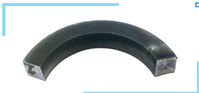
□ Fig. 3.18 Appearance of the sample for plasma precision nitriding Avinit N steel DIN 1.8509
