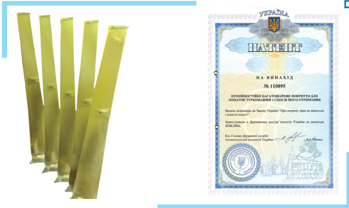
□ Fig. 4.2 Turbine blades with developed protective coating using new complex plasma chemical nanotechnologies and equipment (1.300 mm long)
