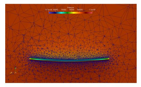
Figure 4.22: Converged aeroelastic solution with CFD solver Su2 and structural finite element solver FramAT  $\,$
