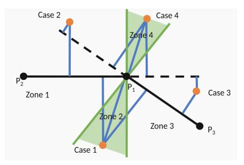
Figure 3.5: Distance computation cases, for moment computation
