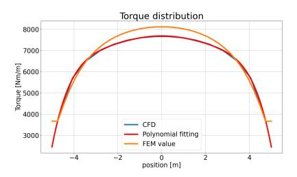
Figure 4.15: Moment distribution, CFD result in blue, polynomial fitting in red
