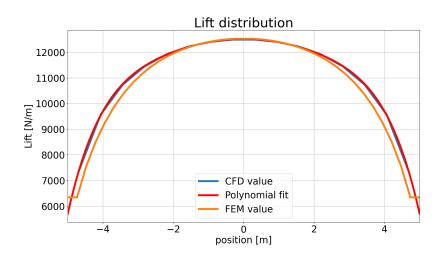
Figure 4.13: Lift distribution, CFD result in blue, polynomial fitting in red, and value found by the radial basis function interpolation matrix.
