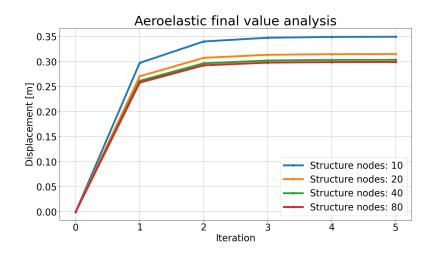
Figure 4.12: Structural mesh total displacement convergence analysis
