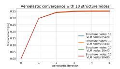
Figure 4.8: Convergence analysis 10 structural nodes
