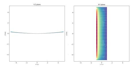
Figure 4.17: Converged aeroelastic solution with VLM solver PyTornado and structural finite element solver FramAT
