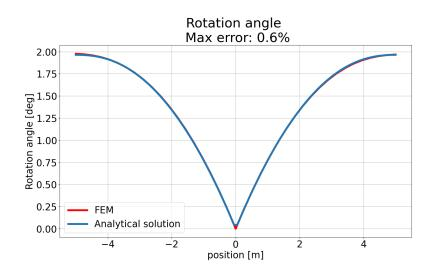
Figure 4.21: Comparison of the rotation angle computed by FEM and by the analytical solution, error computed on maximal displacement
