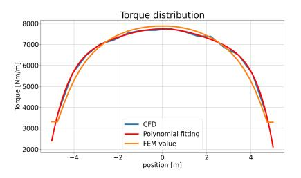
Figure 4.20: Torque distribution on the wing, CFD solution in blue, polynomial fit in red and mapped torque on beam model in orange
