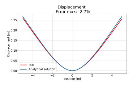
Figure 4.19: Vertical displacement given by FEM, in comparison with the analytical solution, error computed on maximal displacement
