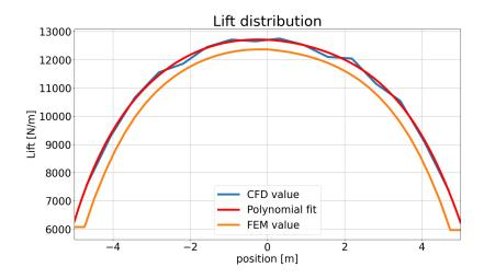
Figure 4.18: Lift distribution on the wing, polynomial fitting, and mapped lift on beam model
