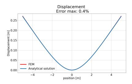
Figure 4.14: Displacement distribution, a comparison between the analytical solution and the finite element beam theory.
