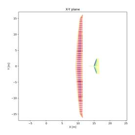
Figure 4.4: Deformed wing (TPS function)
