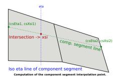
Figure 3.4: Position on a wing for a CPACS file
