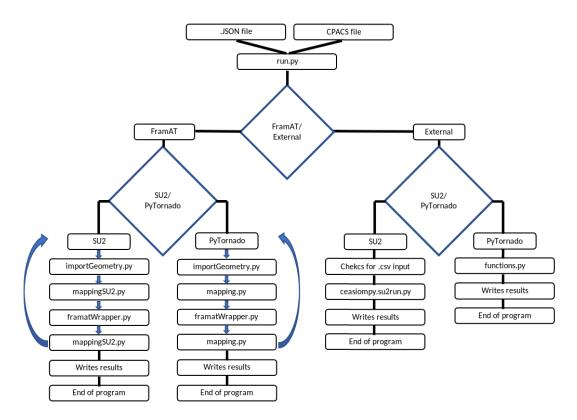
Figure 3.3: Aeroframe 2.0 workflow
