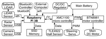
Fig. 2: System dataflow diagram
