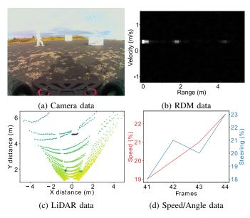
Fig. 3: Frame sample of camera, radar, LiDAR and Speed/Steering data.
