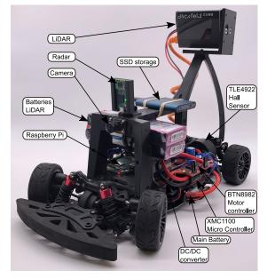
Fig. 1: Developed RC car system
