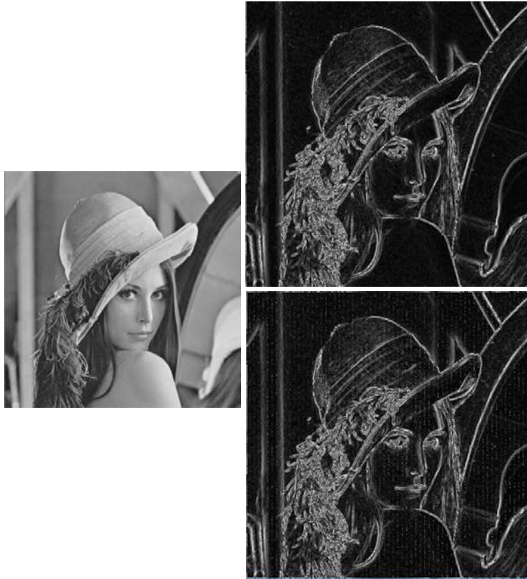
Figure 4.4 Effects of one permanent fault in the control unit of a GPGPU. Original fault-free gray-scale image (left), fault-free edge-detection output image (top-right) and faulty edge-detection output image (bottom-right).
