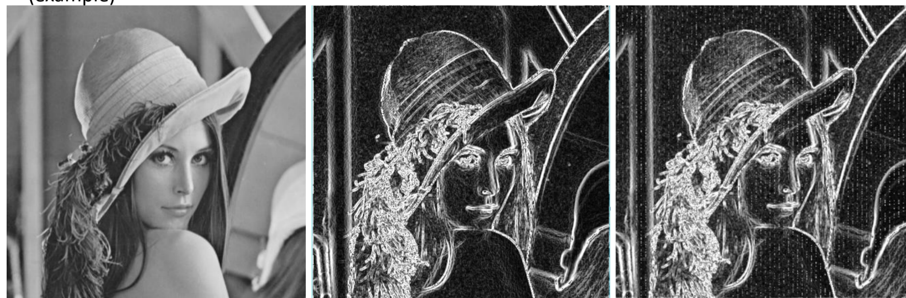
Original Image. Edge detection with Sobel filter. Edge detection result with a permanent fault in SMO actual mask field (Thread 5), 8 threads per block.
