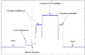
Fig.9 Transmission sensor power consumption
