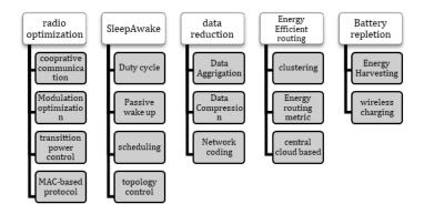
Fig.10 ISO model classification of energy saving techniques
