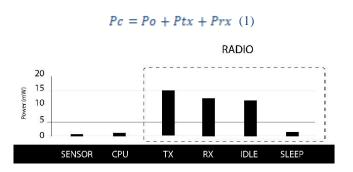
Fig.8 sensor power consumption model
