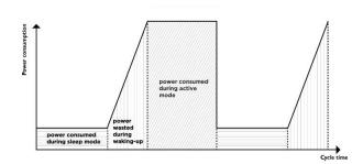
Fig.12 Power wasted during waking up
