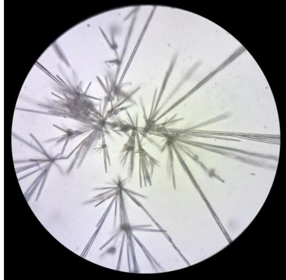
Image 2: Fraction 3, reprecipitated in situ . Now the characteristic needle-shaped harmine crystals can clearly be observed.
