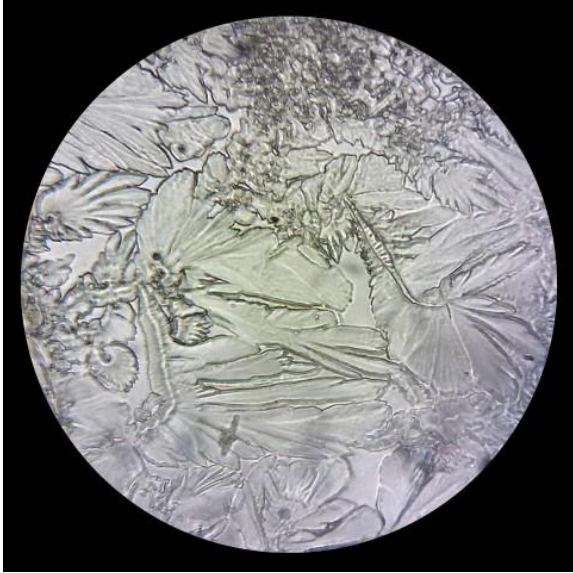
Image 8: Fraction 16: Next to the leaf-like crystals of image 7, other 'floral patterns' can be observed in recrystallized DHH-precipitates.
