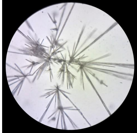
Image 2: Fraction 3, reprecipitated in situ . Now the characteristic needle-shaped harmine crystals can clearly be observed.
