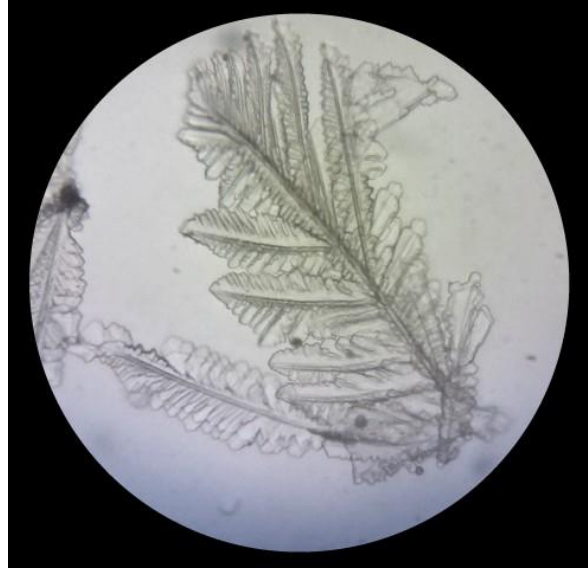
Image 9: Fraction 19: In the last fraction that was precipitated, THH crystals could not be observed next to the remarkable DHH-crystals
