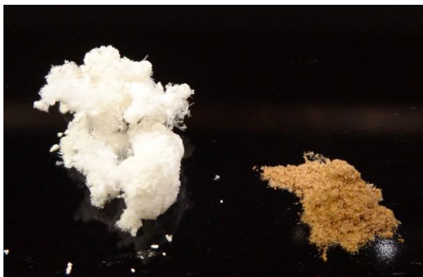
Image 10: A fluffy and snow-white cluster of pure harmine-needles RA7 (left) sublimated from fraction RA2 (right).
