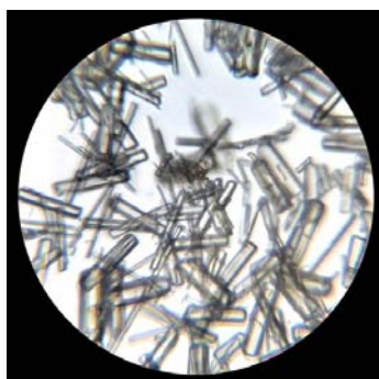
Image 3: fraction 11, showing only the presence of harmine crystals.
