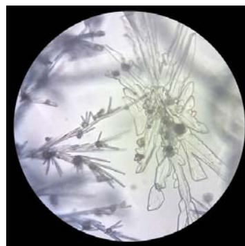
Image 5: the 12th or 'mixed-fraction', recrystallized in situ on the microscopic slide.
