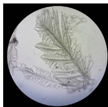
Image 9: Fraction 19: In the last fraction that was precipitated, THH crystals could not be observed next to the remarkable DHH-crystals
