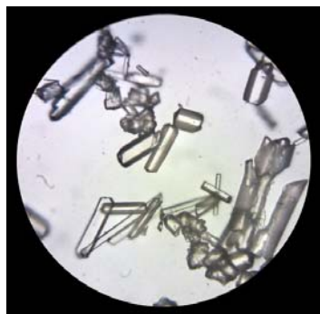
Image 1: Fraction 3: irregularly shaped harmine crystals are formed during gradual basification
