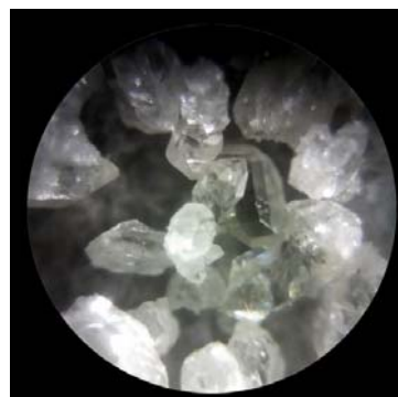
Image 11: Pure DHH prisms (RA5), sublimated from fraction RA4.
