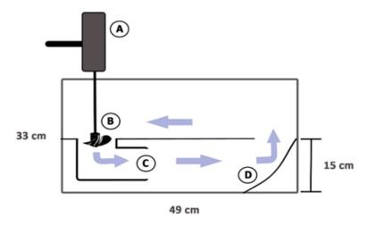
*Figure 4: Experimental 33 flume used to determine feeding rates of the species* Antipathella wollastoni *under different flow rates. A:313 rpm motor; B: 8 cm marine propeller; C: tube facilitating the creation of laminar flow; D: ramp to decrease localized water turbulence. Arrows indicate flow direction.*
