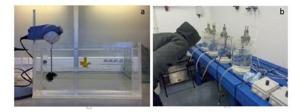
Figure 1: a) Closed recirculation flume (7 L volume) used at the CSM to conduct feeding experiments (Photo:  $\bigcirc$  S. Reynaud), b) Cylindrical flumes (5 L) used for feeding experiments. The motor in the top of the chambers is connected to a blade, which keep the water moving at constant flow speed. The speed of the flow can be switched with the controllers (white boxes in the right part of the image). (Photo:  $\bigcirc$  C. Orejas).
