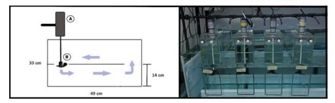
*Figure 5: Experimental 13L flume used to study feeding rates of the two gorgonian species under different flow velocities. A: 113 RPM motor, B: 9 cm marine propeller. Arrows indicate flow direction.*
