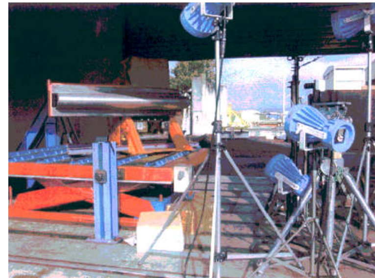
Source: Bird strike testing of leading edge at CEAT / EU CRAHVI
