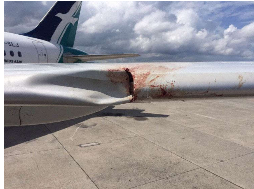
Bird impacted the leading edge of the left hand wing puncturing the leading edge and causing a large dent. The aircraft continued for a safe landing. Source: SilkAir Airbus A320-200. 13.12.2015 on approach to Brunei International Airport
