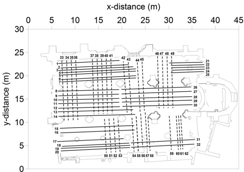
Figure 3 The ERT survey planning inside the Bedestan monument. Full and dashed lines over the sketched topographic map of the complex indicate longitudinal and transversal ERT profile sets, respectively. Table 1 reports the acquisition parameters of each ERT profile.
