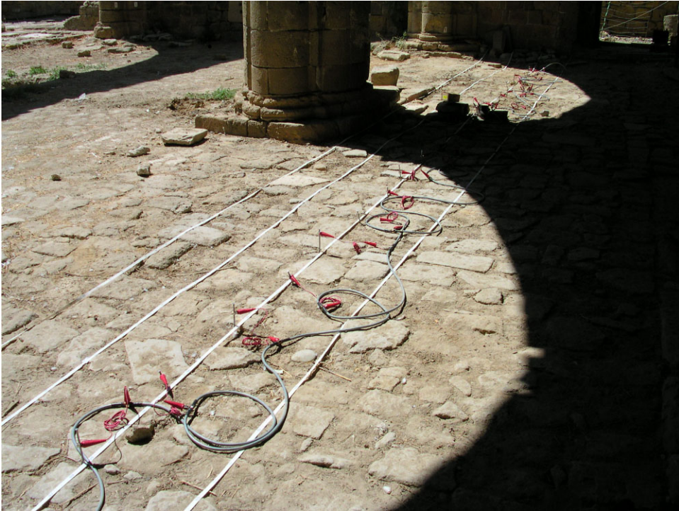
Figure 4 The multi-electrode device spread out on the floor of the Bedestan interior.
